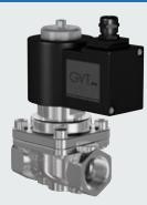
2/2-Way solenoid valve – valve normally closed (NC). When energized the solenoid first opens the pilot hole and then lifts directly or supported by a pressure difference the piston from the valve seat. The valve is closed by spring power.
